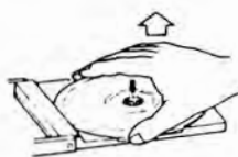
How to remove the disc.
