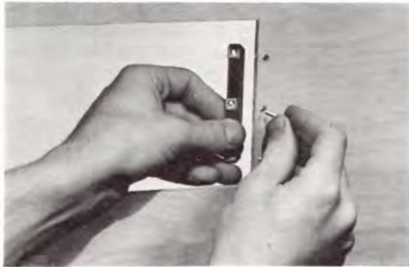
Figure 20. Securing Mounting Strips to Installation Cutout.
