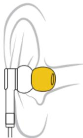
Choose the ear tips that form a seal with your ear canal. Squeeze the eartip, match its orientation to the nozzle, and then press the ear tip against the nozzle to attach.
