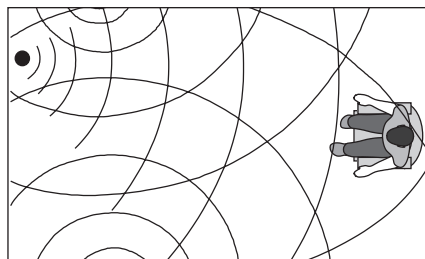
Figure 8-9. As can be seen here, point source concepts invite a great deal of room interaction. While delivering good frequency response to a large listening audience, imaging is consequently confused and blurred.
