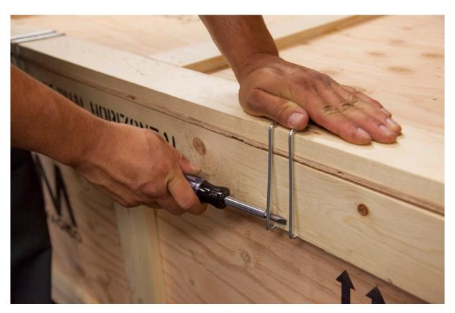
3. Using a flat head screw driver pry away the 6 clips attaching the top of the crate. Do
