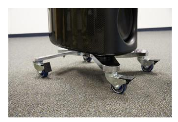
14. POSITION THE M6 IN IT'S DESIRED LOCATION. ONCE IN POSITION, ENGAGE THE BRAKES ON THE (2) REAR CASTER WHEELS. USING THE HELP OF 2 OR MORE PEOPLE, TILT SPEAKER BACKWARD, UNINSTALL FRONT CASTER WHEELS AND INSTALL M-PODS BY CAREFULLY THREADING THEM INTO POSITION.
