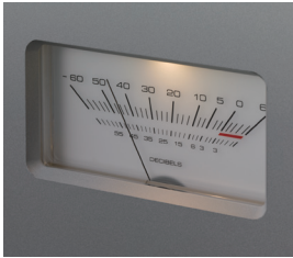
Needle-type meter with electric bulb-colored illumination
