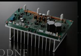
Power amplifier block of parallel module ODNF version 4.
