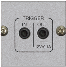
12 Volt trigger input / output terminal Powering on and off compatible devices can be achieved via connections over a commercially available 3.5mm monaural mini jack cable.
