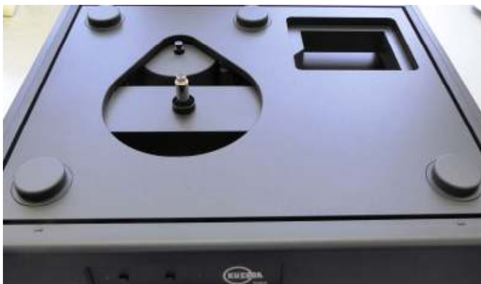
Fig. 3. Top plate in the outer frame with 4 height knob adjustments
