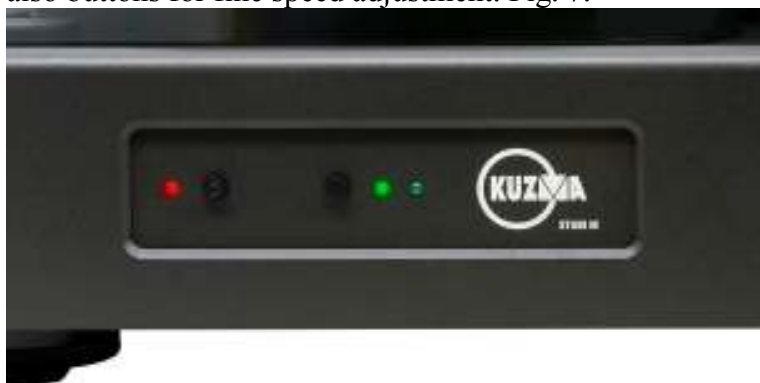
Fig.7. Front panel: Left- Start/Stop, Right- Speed Selection ( left LED 33, right LED 45 )
