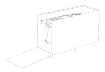
Unscrew the top cover of the crate and remove to top cover. By unscrewing the crate at the bottom side of the speaker, a ramp will be created to be able to pull the speaker out of the crate.
