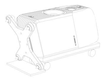
Step 4: Guide the speaker to its final position Tilt the speaker and leave the cart on the ground.
