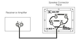
IMPORTANT: Do not reverse polarities (i.e., "+" to "-" or "-" to "+") when making connections. Doing so will cause poor stereo imaging and diminished bass performance.
