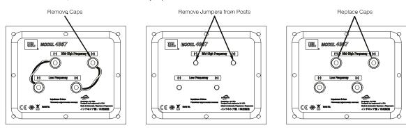
If you're bi-wiring with a single stereo power amplifier, connect the speakers according to the following illustration.
