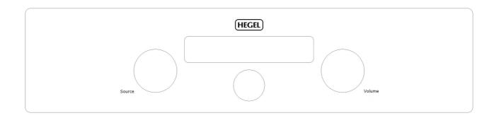
The H100 amplifier is switched on with the power button in the middle of the front panel. Blue color characters in the display indicates that the amplifier is switched on.
