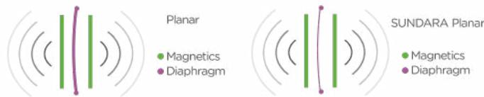
Compared to conventional dynamic drivered headphones, planar magnetic headphones have solved problems such as surface distortion of high frequency audio and the lingering vibrations in a dynamic loud-speaker. The large and heavy magnets used face a residual vibration due to the retained momentum in the driver as it moves. In a Planar Magnetic the utilization efficiency has been improved by the weight of drivers being reduced with the use of our ultra-fine diaphragm in the SUNDARA.
