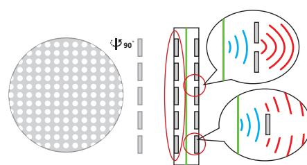
A conventional dynamic driver's frequency response can be altered due to distortions and vibrations across the diaphragm surface.
