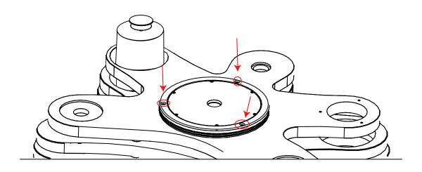
**STEP 17-3**Remove the Platter Flange as indicated in the picture aside
