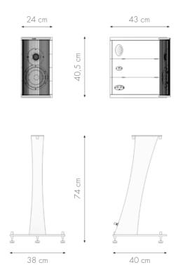
Frequency Response: 39-23000Hz Nominal impedance: 7 ohm, minimum 3.8 ohm at 5500hz Sensitivity: 2.83V1m:87 dB
