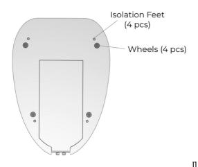
Then screw the isolation feet into the specific holes as shown in drawing 12.
