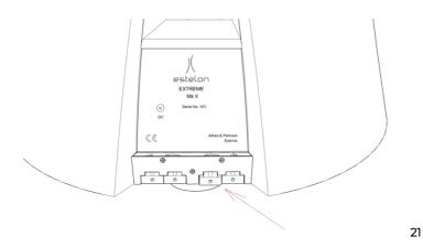
**NB!** When connecting the speaker to the amplifier please make sure that the amplifier is in the off position. Connect the speaker cable to
