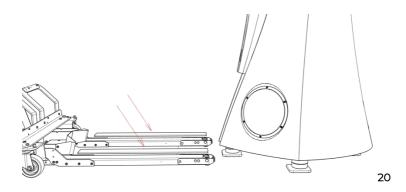
4. Lift the speaker again making sure that the lift cart has 125 mm (4,9") free space from the front part of the speaker. Remove the base spacers and screw in the spikes as shown in drawing 21.
