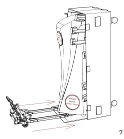
8. Take the hand lever and insert it into the lift cart. Then turn it 90 degrees clockwise, as shown in drawing 8.
