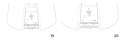
In order to exchange the 2-wire connector bridge, with the 4-wire connector bridge which is included in the accessories box, you will need to remove the 3 screws of the attached bridge connector with the use of a PH1 tip screwdriver (not included) and replace it with the 4-wire bridge connector.
