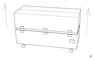
5. Remove the accessories box and the cover plates box from the flight case. (drawing 4)
