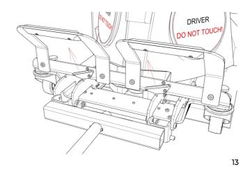
15. Lift the lever so the lift cart forks release the speaker. (drawing 14)
