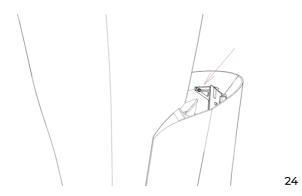
When pressing the switch up, the upper module of the speaker will move up, and when pressing the switch down, the upper module of the speaker will move down.
