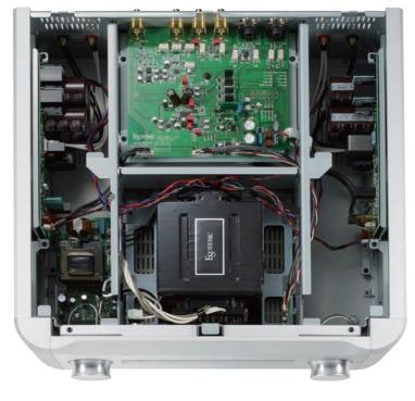
supply. This design assures low noise operation with a complete shutdown of the control microcomputer except at the time of receiving an operation request.
