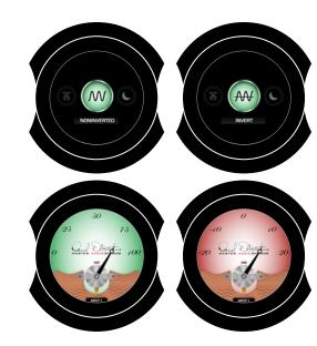
red when the polarity is inverted. Depending on the recording, the effects of polarity inversion are often subtle and sometimes even inaudible. The display will alternate between the two different icons to indicate polarity status.
