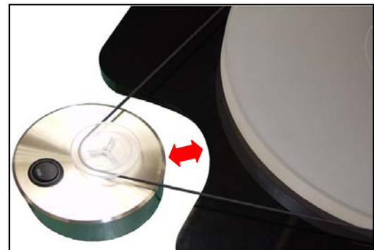
5. Place the pulley on the motor spindle. The distance between the pulley and the motor housing should be approx. 1-2mm. Tighten the little screws inside the pulley with the aluminium screwdriver provided.
