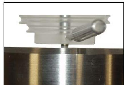
6. Place the belt first round the platter, then round the smaller diameter of the pulley (33 1/3 rpm).
