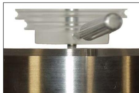
4. Take the motor and place it in the indent of the chassis. The switch should be on the outside of the turntable and the space between motor and chassis approx. 1cm
