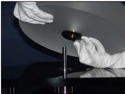
**Picture 1:** Placing the platter
