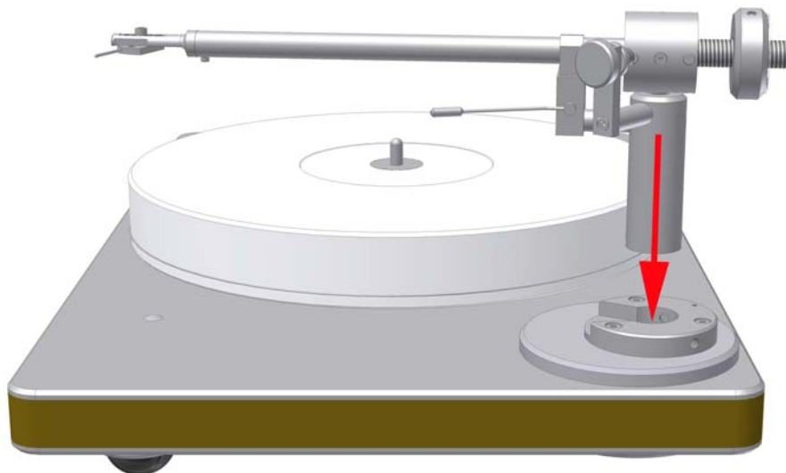
Pic. 17: Mounting the clearaudio Satisfy tonearm
