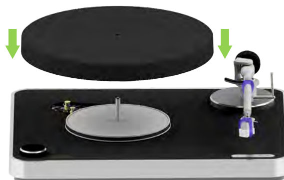
Pic. 4: Placing the platter
