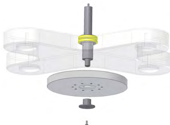
Pic. 15: To insert the bearing spindle into the bearing sleeve
