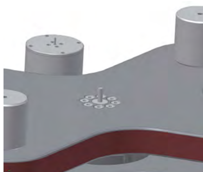
Pic. 11: Tighten the bearing screws
