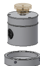
Picture 19: Positioning the motor- unit into the stainless steel motor stand
