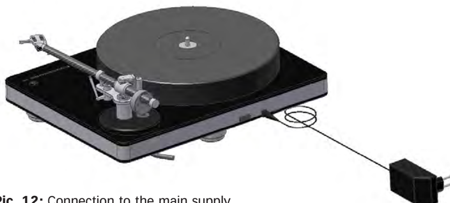
Pic. 12: Connection to the main supply
