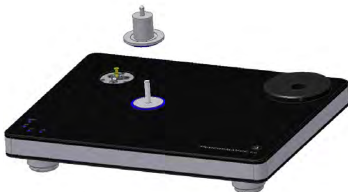
Pic. 6: Fitting the bearing upper part
