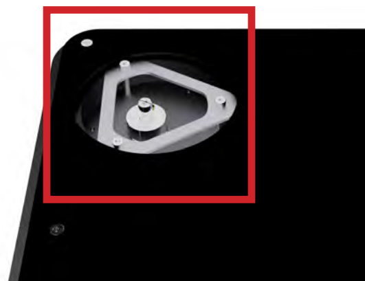
Pic. 10: Adjustment of the anti-skating
