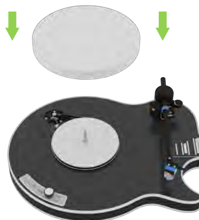
Pic. 5: Placing the platter
