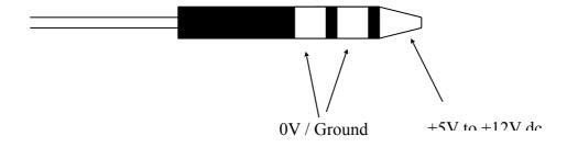
The tip of the plug is the +5V to +12V dc connection, the centre and rear connection are the 0V or ground connection.
