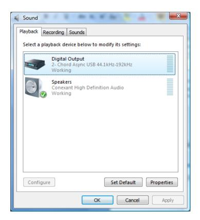
It is also a good idea at this stage to set the Digital Output as the default sound output device. Highlight Digital Output as shown then click the Set Default button at the bottom of the page. Click the OK button to continue.
