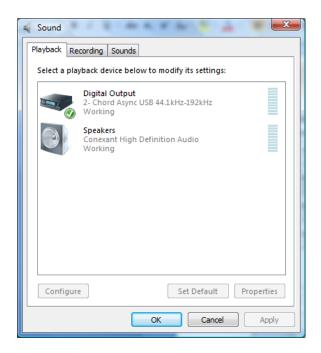
Here you have a list of the connected audio devices. The QBD76 HD is identified as a digital output device with the 'Chord Async USB 44.1kHz-192kHz' driver installed. Shown at the top of the list here. Right click the digital output and select properties to show the following screen:-
