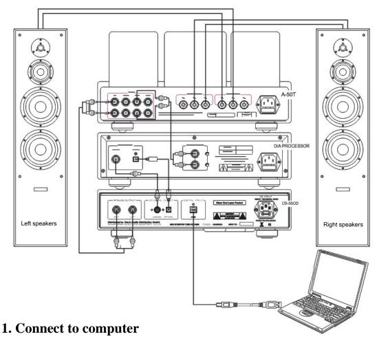
Connect the USB port to the computer's USB port with the USB cable which must be according to the USB2.0 specification. Only the USB port in the rear panel can be used for desktop computer.
