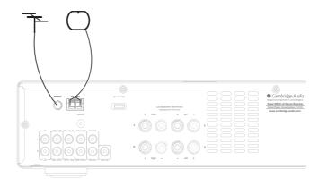
**Note:** The SR10 is supplied with a temporary aerial for initial use. For permanent use, outdoor aerials are highly recommended.
