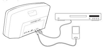
When the Minx Air is not streaming audio from Bluetooth, Airplay or Internet radio is automatically selects the analog audio inputs for playback.
