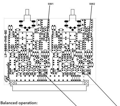
For balanced operation (BAL) the switches **B\_L** (left channel) and **B\_R** (right channel) must be switched to BAL position.
