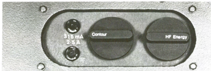
Location of protective fuses (front grilles removed)
