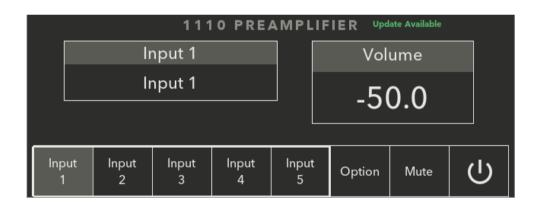
The 1110 has a large, centrally mounted display located between the buttons and control knob. There are **8** buttons that will each correspond to various functions, depending on whether the unit is showing the Home Screen, Option Screen, or Setup Screen.
