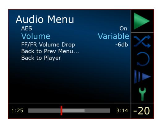
If the 1021 will be connected directly to an amplifier, the volume control mode should be set to **Variable**.
