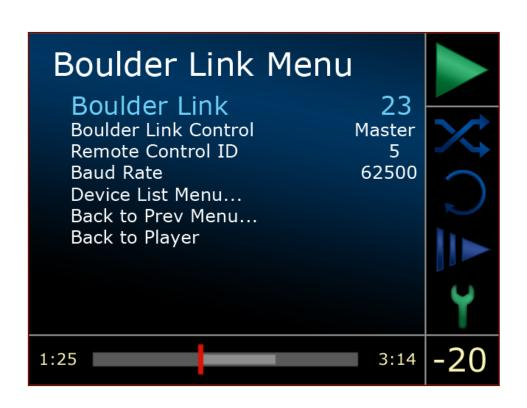
The Baud Rate submenu can be set to **4800** or **62500**. The default setting is **62500**. To select a baud rate, use the **Navigate Left** or **Navigate Right** button to select a specific rate. Consult your dealer before changing this setting.
