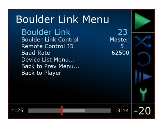
The Boulder Link ID can be set for values of **16 through 31**. To select an ID number, use the **Navigate Left** or **Navigate Right** button to select the specific ID number you prefer.
