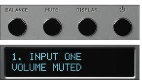
To temporarily reduce the volume, press the MUTE pushbutton. "VOLUME MUTED" will show in the display, replacing the volume indication. Again pressing the MUTE pushbutton will return the volume to normal level.
