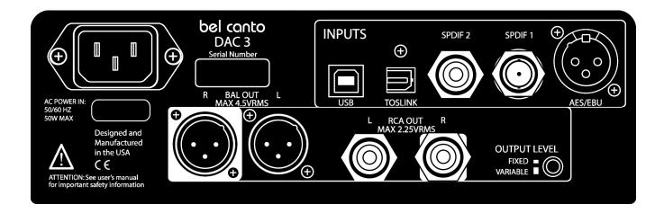
IMPORTANT: If using the DAC3 directly into a power amplifier, ensure that the Fixed/Variable Output button is in the OUT (variable) position. Operation in Fixed Mode directly into the amplifier could cause extreme output levels, clipping and damage to the loudspeakers, amplifiers or your ears!
