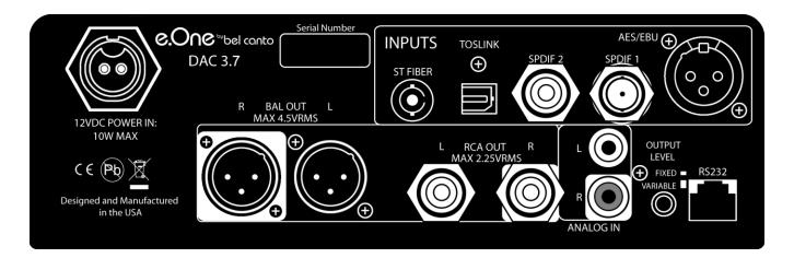
IMPORTANT: When using the DAC3.7 directly into a power amplifier, ensure that the Fixed/Variable Output button is in the OUT (variable) position. Operation in Fixed Mode directly into the amplifier could cause extreme output levels, clipping and damage to the loudspeakers, amplifiers or your ears!
