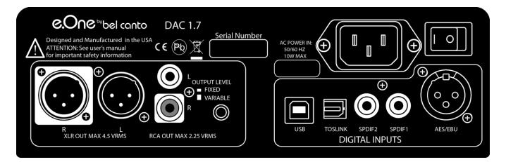
IMPORTANT: If using the DAC1.7 directly into a power amplifier, ensure that the Fixed/Variable Output button is in the OUT (variable) position. Operation in Fixed Mode directly into the amplifier could cause extreme output levels, clipping and damage to the loudspeakers, amplifiers or your ears!
