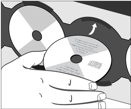
The CD must be loaded with the text side facing you. Hold the CD by its edges and insert the CD (top section). To unload the CD, hold it by its edges and push the CD slightly forward to release it.
