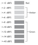
The color-coded front panel bar-graph displays how much of the available digital range is being used. The uppermost segment is red and indicates that clipping has occurred (with a display hold time of ten seconds).
