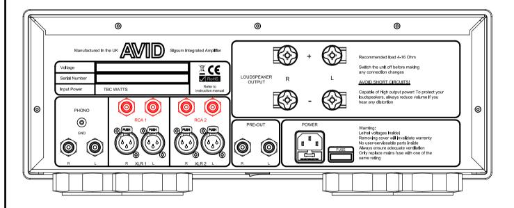
The Sigsum has Four line inputs: two Balanced and two Unbalanced— which you choose depends on your source equipment, but if you have the choice, we recommend using Balanced. These are referred to as Line Level inputs, and can be used to connect to any standard piece of audio equipment, such as CD, Media Streamer, or FM/DAB Tuner.
