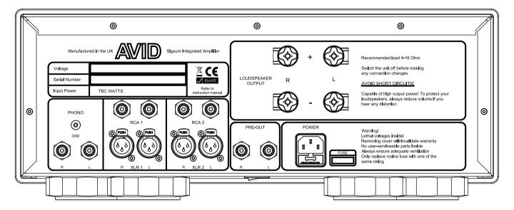
Your **AVID** amplifier can make use of a either <u>Balanced</u> (XLR), <u>Unbalanced</u> (RCA), or any combination of the two types of input.
