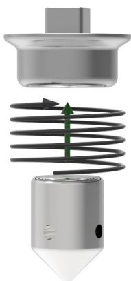
Screw spike into shroud
