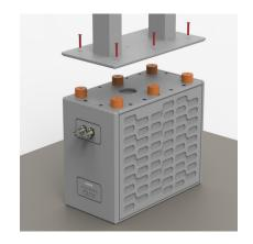
**10** Once the stand is correctly located, attach the stand securely using the six 40mm M6 bolts removed in step 1.
