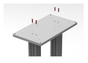
**4** Using the supplied 25mm countersink bolts (D), attach the two pillars (B) to the base of the speaker stand (A).
