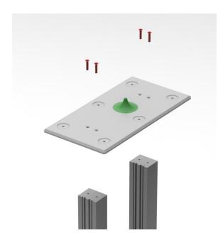
Take the plinth you previously removed from the loudspeaker and bolt it to the top of the pillars (ensuring that the anodised deflector is pointing upwards), using the four 15mm M6 bolts (C) supplied. Ensure they are done up tightly—there should be movement between the plate and the pillars.
