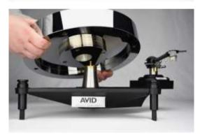
Gently and gradually place the platter onto the main bearing, ensuring that the spindle does not come into contact with or leave any scratches on the tapered bore in the platter.
