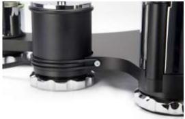
After positioning the motor in place, secure it to the main chassis using the rubber O-Ring provided. Stretch the O-Ring around the motor, fastening each end to the bolt heads on the side of the main chassis.
